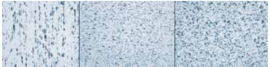
AgC3 longitudinal section (parallel to the direction of extrusion)
