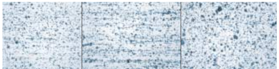
longitudinal section Ag/SnO 2 92/8 SPW
