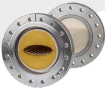
Kicker chamber Ø 150 x L 300 mm with TiN coating made of FRIALIT F99.7
