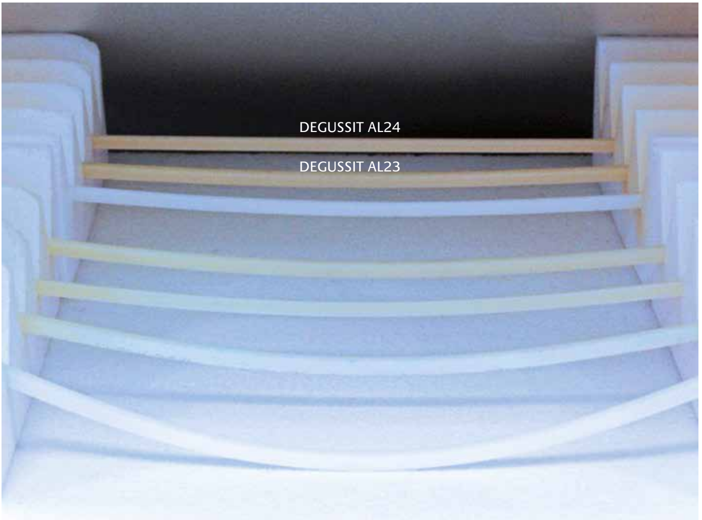
Comparative test used to determine \text{Al}_2\text{O}_3 high-temperature strength
